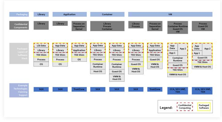
As can be seen in the diagram, each of these nine embodiments can be mapped to one of the four aforementioned packaging terms. The red boxes show the set of components running inside a TEE. The yellow boxes show an example of what might be packaged together. In another example (not shown) some of the components inside a red box might be packaged separately.
